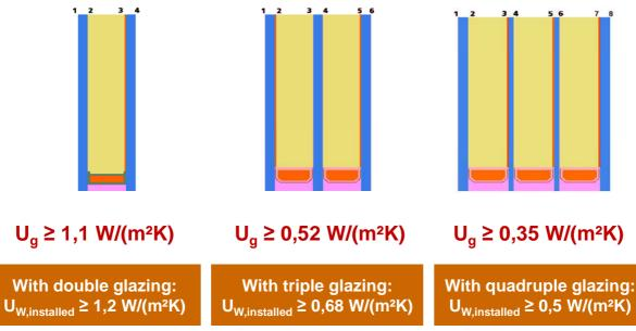
Figure 4: Achievable U-values of the installed window.
