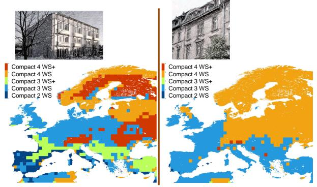
**Figure 11:** Types of windows and glazing in the economic optimized building under based on possible future price levels or quadruple glazing.
