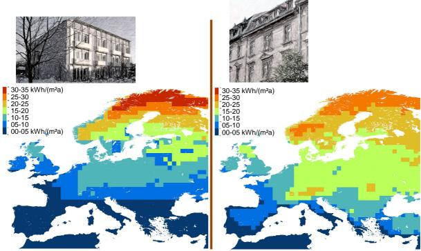
Figure 7: Heating demand of the cost optimized buildings.
