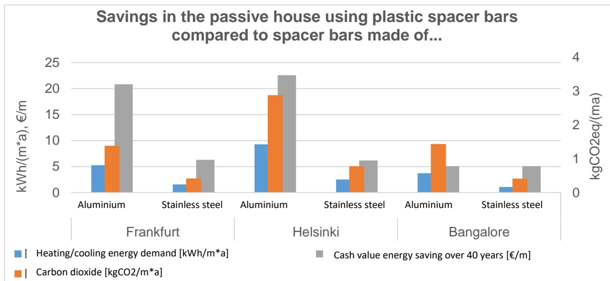
**Figure 4:** Savings in the passive house building model per linear metre of glass edge
