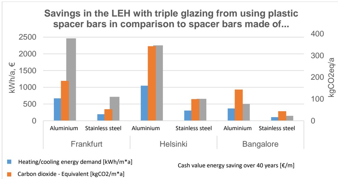
**Figure 8:** Savings in the triple glazed low-energy house building model
