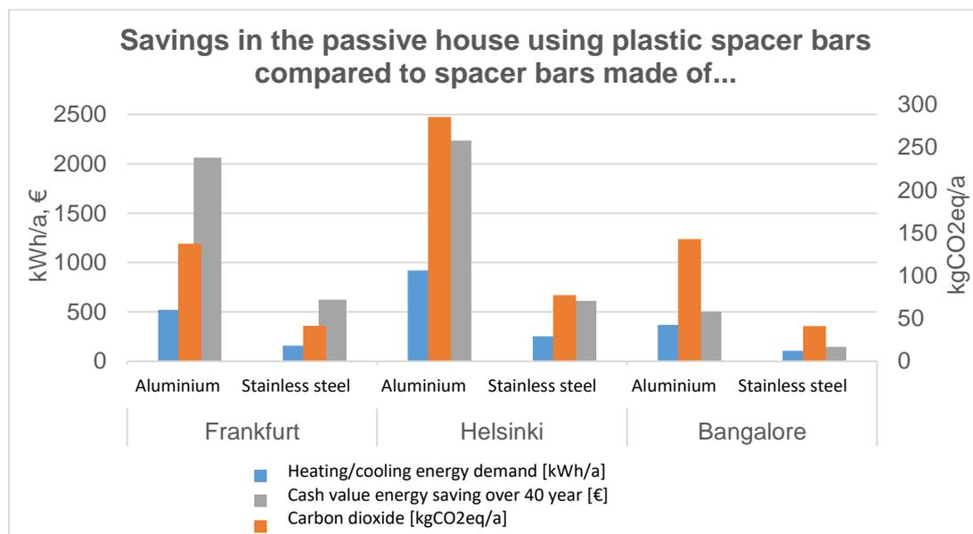
**Figure 3:** Energy, cost and CO<sub>2</sub> savings in the Kranichstein passive house building model
