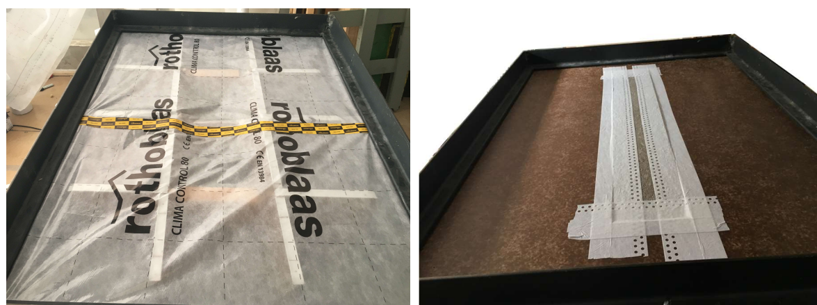
Figure 1: Test setup surface sealing. Left case 1 (table 2), right case 3 (table 2), tentative
