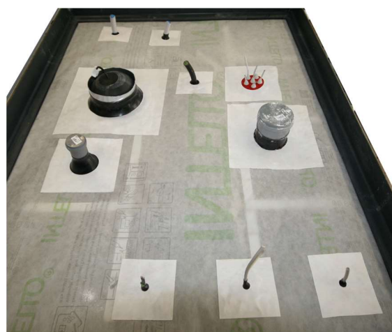
Figure 3: Test setup for penetrations in membrane, tentative
