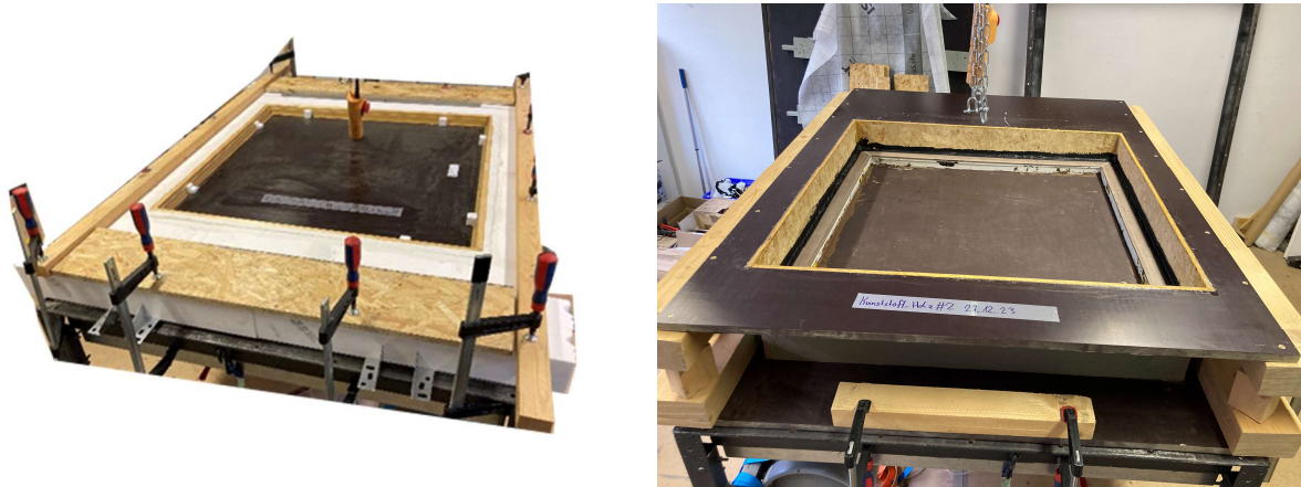
Figure 2: Test setup window connection. Left wooden frame in front-of-wall installation system on concrete wall, right plastic frame in framed wall, tentative
