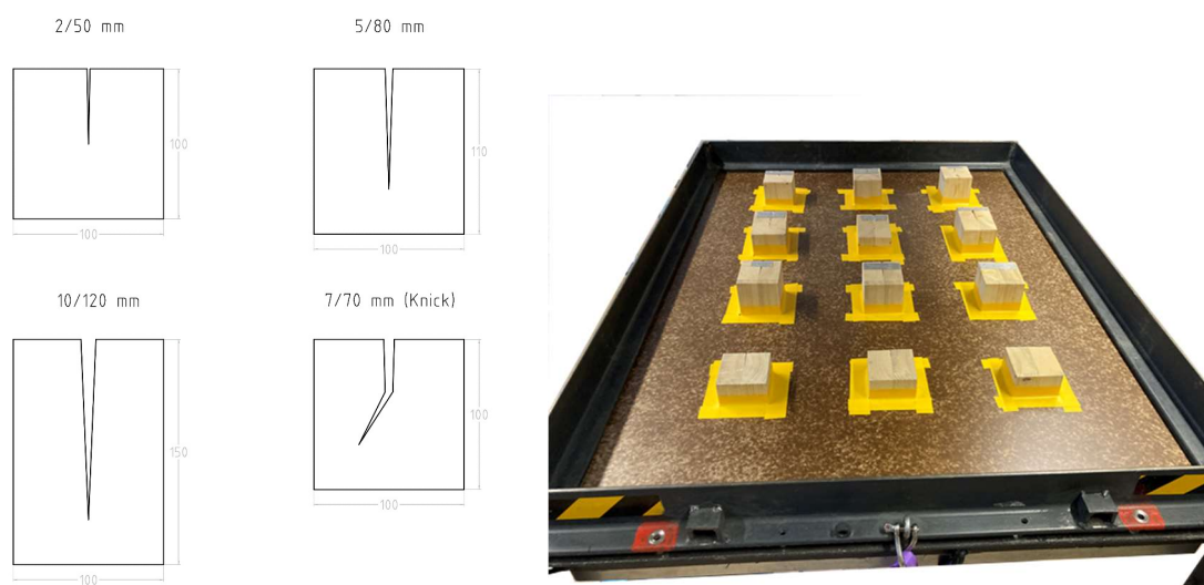
Figure 4 left: Specimen blocks with different artificial shake geometries. Right: Test setup wooden beam sealing, tentative
