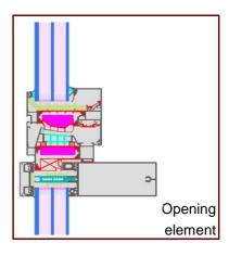
\* Spacers of lower thermal quality lead to higher thermal losses and lower glass edge temperatures.
