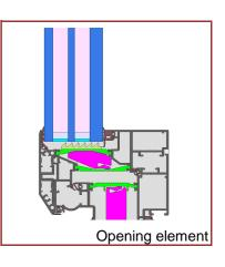
\* Spacers of lower thermal quality leading to higher thermal losses and lower temperatures.
