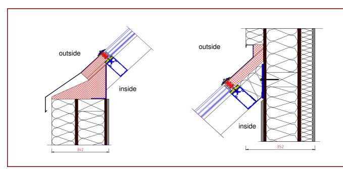
Installation based thermal bridge  $\Psi_{\mbox{\tiny install}}$  in Passive House suitable walls
