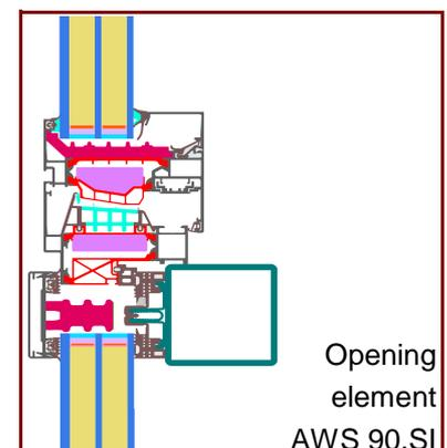
\* Spacers of lower thermal quality leading to higher thermal losses and lower temperatures.
