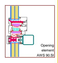
\* Spacers of lower thermal quality leading to higher thermal losses and lower temperatures.
