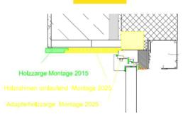
step is fixed to the one already installed, and a CompacFoam frame is fitted on the outside. The window is refitted and the EIFS is applied. The roller shutter box is flush with the wall also in the new position. The *System Connecta* was developed as a universal adapter for all Optiwin window systems and is also suitable for other windows.
