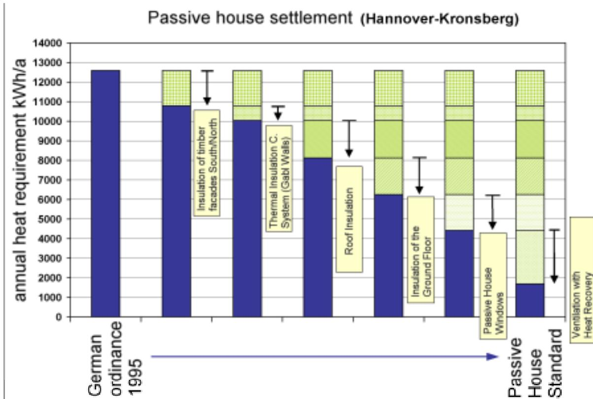
**Figure 26: Six steps from the insulation ordinance standard to the Passive House: Through the energy efficiency measures described in the text, the yearly heating energy requirement (incl. building services losses) is reduced by more than 80%. The Passive House standard on the far right was realised in the Kronsberg built estate.**
