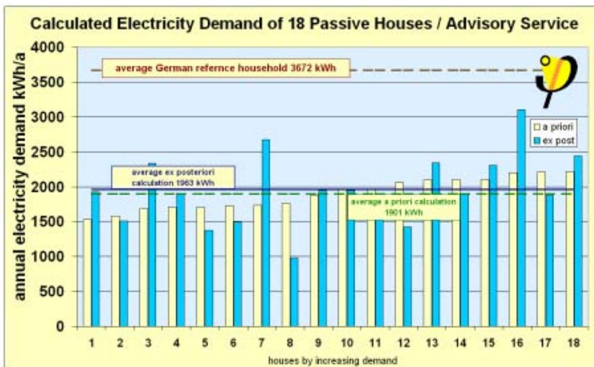
Figure 70: Comparison of a-priori and ex-posteriori calculations of the annual electricity demand for 18 households in the Hannover Passive House estate
