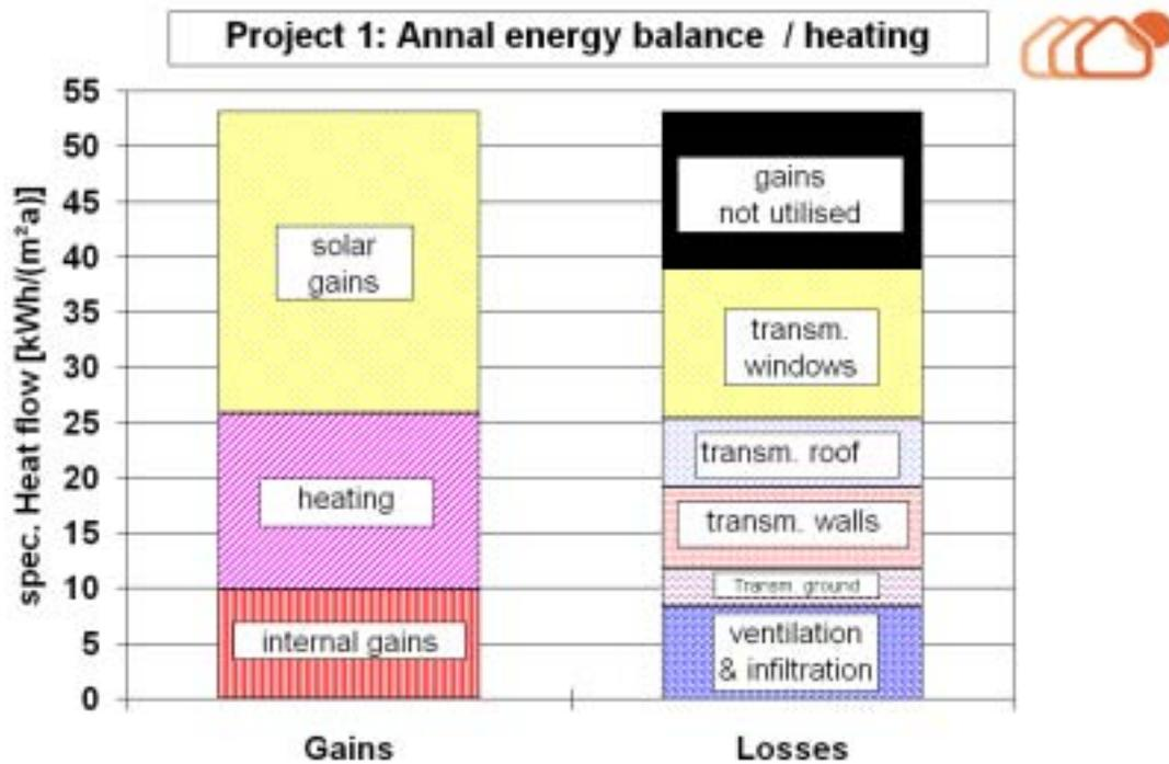
Figure 45: Annual heating energy balance in the first measurement year (01.10.1999 to 30.09.2000).
