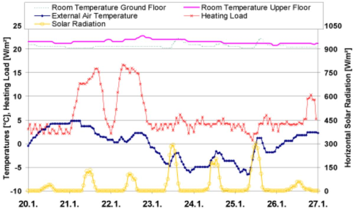
Figure 58: A typical cold and sunny week in winter, during the first heating period 1999/2000
