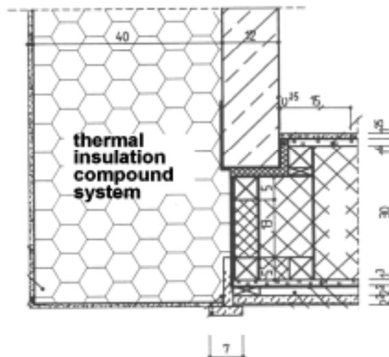
Figure 13: Junction of the facade element and the gable wall
