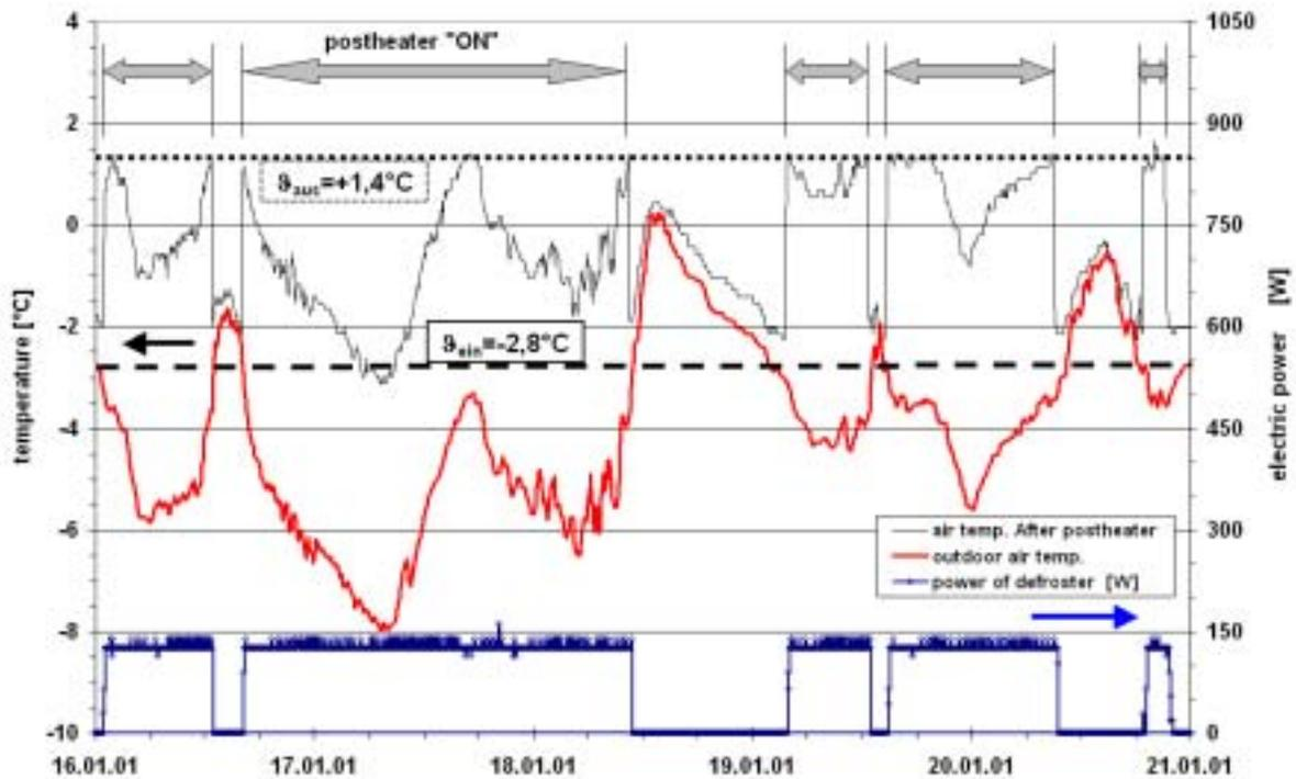
**Figure 77:** Operation times of the electrical frost-protection device (on and off temperatures), which is placed in front of the ventilation system's heat exchanger. Data from the 16<sup>th</sup> to the 21<sup>st</sup> of January 2001 is shown. The electrical output of the heater defines the operation times. The turning on temperature equals an outdoor temperature of -2,8 °C, the switching off temperature equals a temperature of +1,4 °C behind the device.
