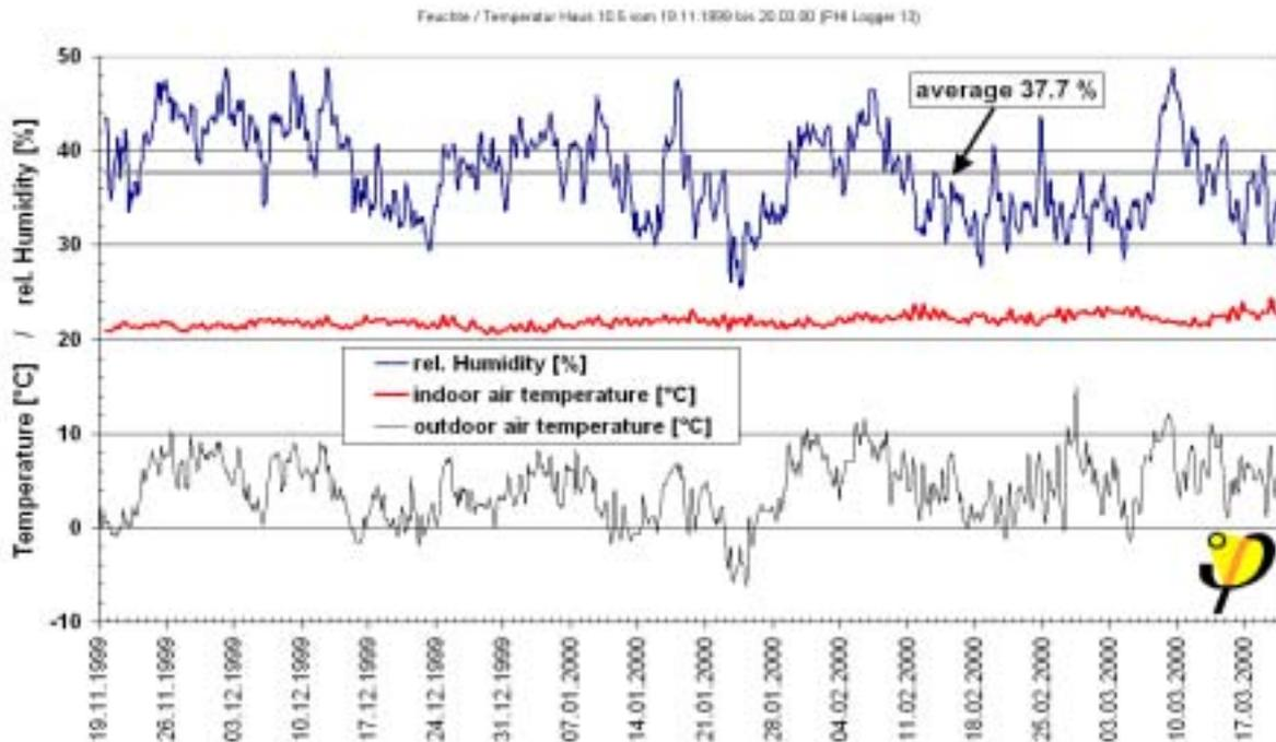
**Abb. 78:** Relative room air humidity and air temperature in the ground floor living room of a Passive House as well as the outdoor temperature evolution from 19.11.1999 to 20.03.2000. The stand alone data logger recorded the data from the building at 2-hour intervals. The floating averages of four data points are presented.
