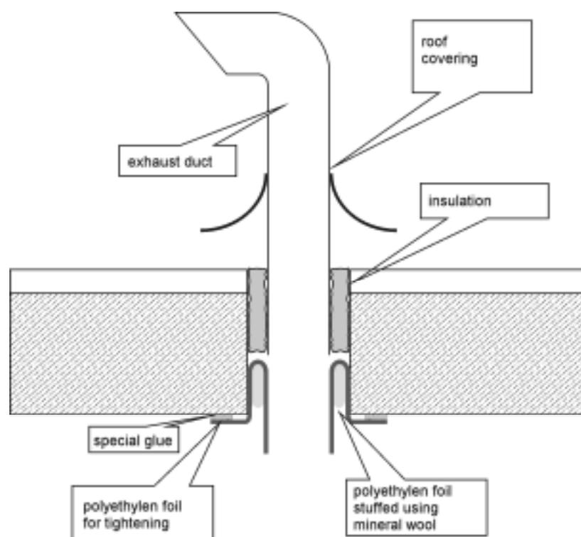
Figure 32: Airtight ventilation duct penetration in the roof area.
