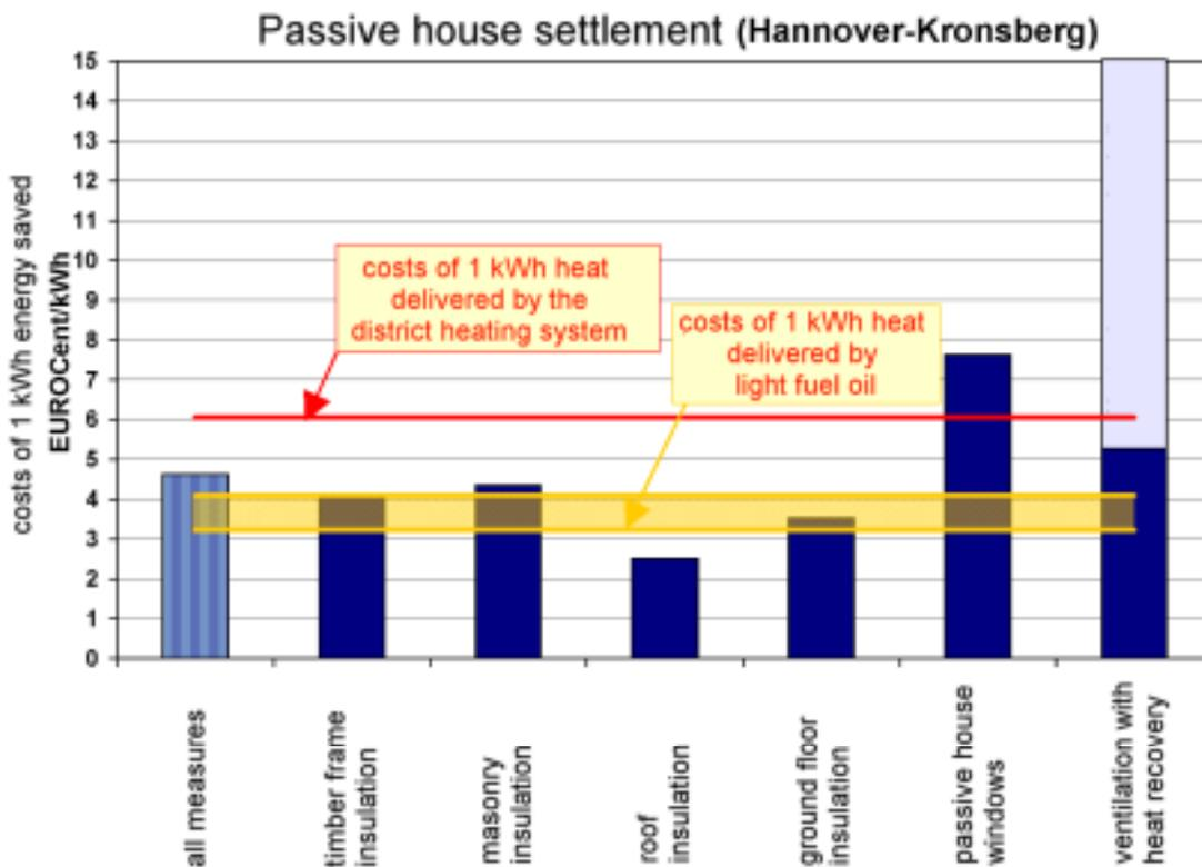
Figure 28: Costs for the „saved kilowatt-hour“ due to the efficiency measures in comparison to the district heating supply and the end energy price for heating oil in Germany. The left column is the sum of all measures (WSVO-standard → Passive House standard), the rest for the respective additional measures of the individual steps.
