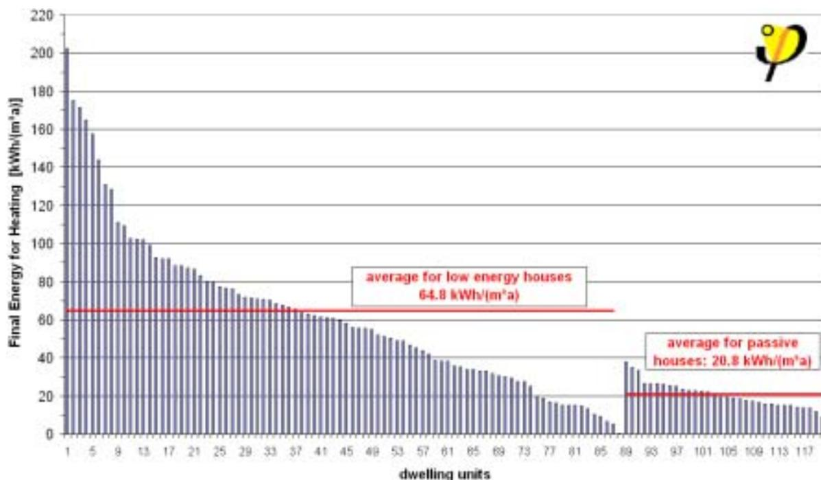
**Figure 52: Comparison of the final energy demands for heating of five Kronsberg multi-family houses built to the Low Energy standard (according to the heating bill) and of the 32 Passive Houses. The comparable annual periods of one year are presented (LEH: 15.10.1999 to 16.10.2000, PH: 01.10.1999 to 30.09.2001). The average of the measured values clearly shows the difference between the two standards.**
