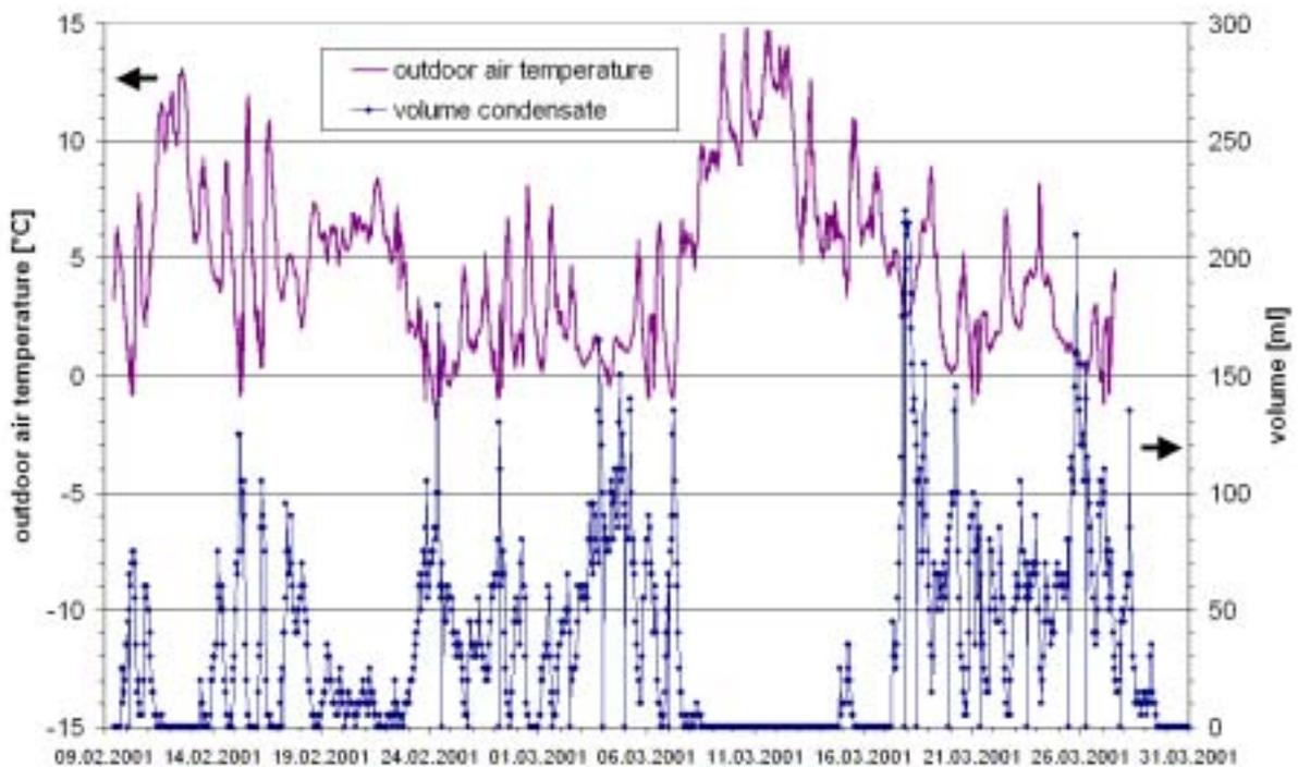
Figure 76: Condensate volume in the heat recovery system in comparison to the outdoor air temperature (temperature: hourly average, condensate: hourly sums).
