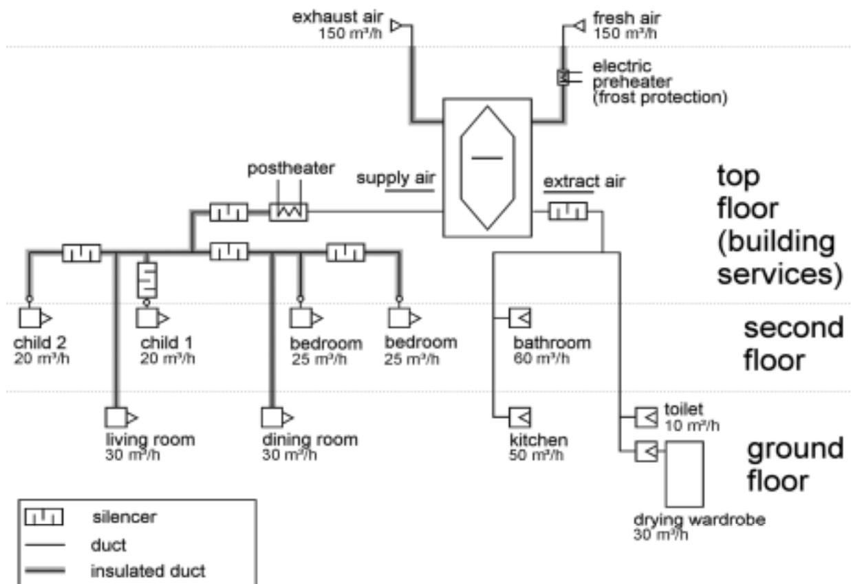
Figure 18: Ventilation system duct network plan for Passive House type „Jangster de L x“ with the design layout flow volumes
