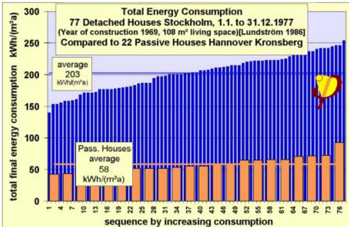
Figure 53: Comparison of the final energy consumption for heating, hot water and household electricity in the 22 permanently occupied Passive Houses with the 77 Stockholm houses according to [Lundström 1986].
