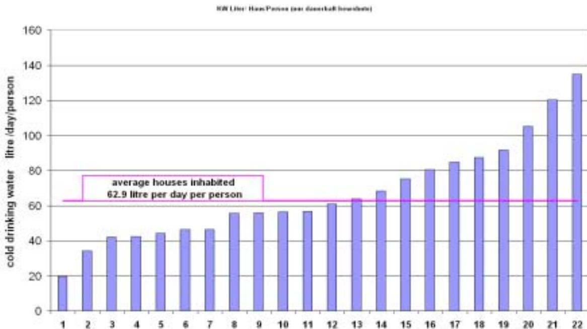
Figure 66: Average cold water consumption amount per day and person in litres from 01. October 1999 to 30. September 2000 for the 22 permanently occupied houses.
