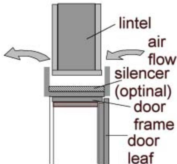
Figure 20: Overflow openings between the lintel and the door frame (source ebök)
